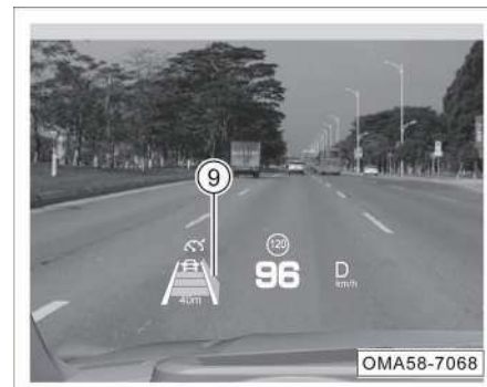
⑨ Red warning belt: BSD triggered
