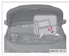
Engine model and serial number as arrowed is located on the engine block (above the starter mounting location).
