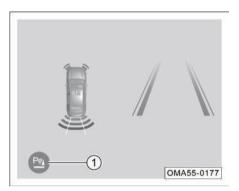
When the RPA is turned on during reversing, press  $P_{\text{WA}}$  the button ① on the AVM interface to manually turn off the system, and press it again to turn on the system. The RPA will be turned on automatically after the vehicle is restarted.
