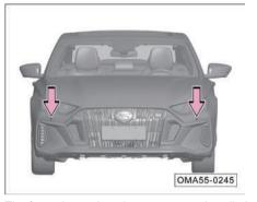
The front ultrasonic radar sensors are installed on the front bumper cover. (for models with vertical grille\*)
