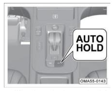
When the engine is started and the driver's seat belt is fastened, press the AUTO HOLD button, the button indicator lamp illuminates and the AUTO HOLD is turned on. Press this button again. The button indicator lamp goes out, and the AUTO HOLD is disabled.
