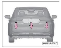
The rear ultrasonic radar sensors are installed on the rear bumper cover. (for models with vertical grille\*)
