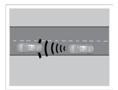
Second-level braking: Slight automatic emergency braking is applied if the ego vehicle continues to approach the lead vehicle.
