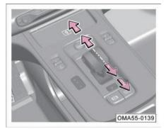
The gears of the gearshift lever are " P, R, N, D, M\* ". When the power supply of whole vehicle is in "ON" gear, the corresponding gear information should be displayed on the instrument cluster after the gear is switched.
