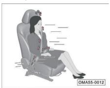
The seat belt pretensioner and load limiter can reduce the pressure of the seat belt on the chest of the driver or passenger and improve the protection performance.
