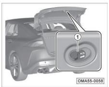
When the vehicle is out of power or the trunk lid fails to be opened normally, you can try the emergency interior opening of trunk lid:
