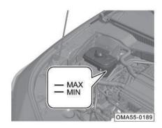
Check whether the coolant level in the intercooler coolant expansion tank is between the maximum scale mark "MAX" and the minimum scale mark "MIN".
