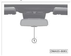
The auto dimming interior rearview mirror monitors the light in front and rear of the vehicle according to the light sensor, and reduces the glare reflected off the rear to the mirror surface, thus realizing the optimal rear view.
