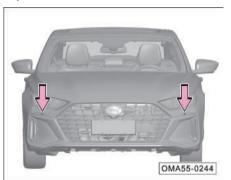
The front ultrasonic radar sensors are installed on the front bumper cover. (for models with transverse grille\*)
