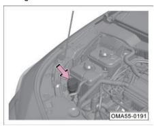
If the level of the washer fluid is too low, the washer fluid shall be added in time.
