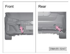
Pry off the towing hook cover in the arrowed position using a slotted screwdriver wrapped with a cloth.
