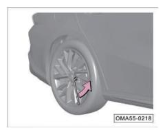
Set the wheel bolt removal wrench firmly on a wheel bolt, and unscrew the wheel bolt counterclockwise.
