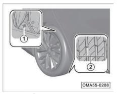
The mark ① is used to indicate the wear condition of the tire outer circle pattern. If the tire outer circle pattern wears to the condition as shown, the tire can no longer be used safely and must be replaced immediately.
