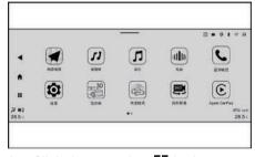
Click the menu key in the system navigation bar on the left side of the desktop to enter the system detailed application menu interface, click the driving mode icon to enter the driving mode application interface, and click the soft button to select driving mode.
