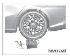
Screw the fitting of the inflator pump into the tire valve, during which a slight air leak will be heard and it indicates that the air passage between the pump and tire has been established. In this case, go on screwing in the fitting.
