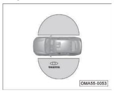
When the intelligent active unlock function is activated and the intelligent remote control key is within 1 meter from the vehicle, the vehicle will be automatically unlocked and the exterior rearview mirrors\* will be automatically unfolded.
