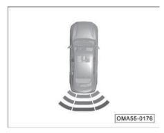
The dynamic view appears at the upper left of the display screen, indicating the distance between the rear of the current vehicle and the obstacle. In the view, the outermost sector is green, the middle and innermost sectors gradually turn to yellow and red. When the vehicle is getting closer and closer to an obstacle detected, the colorful sectors will come nearer and nearer to the car icon.
