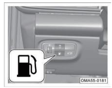
Press and hold the fuel tank cap opening button to make the fuel tank cap pop up.
