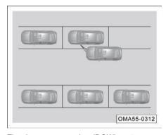
The door open warning (DOW) system uses the BSD sensor installed at the rear of the vehicle to detect the adjacent lane during parking, and when another vehicle is detected approaching quickly and will cause risk of collision if the door is opened, alerts the driver via the visible signal on the exterior rearview mirror and the audible alarm.
