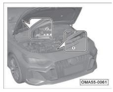
Lift the hood up to the limit position, take out the stay bar from the stay bar bracket ①, and fix the stay bar in the fixing hole ② to support the hood at the limit position.
