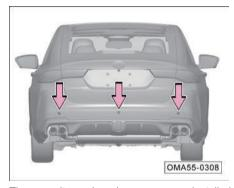
The rear ultrasonic radar sensors are installed on the rear bumper cover. (for models with transverse grille\*)
