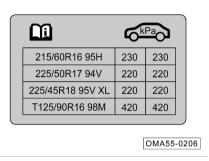
The standard tire pressure data label of the original tire of this vehicle is attached to the B pillar on the driver's side.
