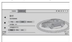
After entering the driving mode interface, click Current Mode Settings to enter the driving mode settings to set the system parameters under the current driving mode:
