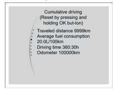
Cumulative driving: It indicates the driving information (cumulative distance/ average fuel consumption/ driving time) of the vehicle since the last reset, which can be reset by pressing and holding "OK" button. The odometer information is displayed on this interface and cannot be reset.
