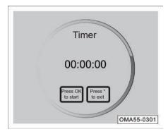
The timer can be activated with the custom button. The timer function can be activated via the steering wheel custom button when the custom button is set to perform the function of the timer through the center console.
