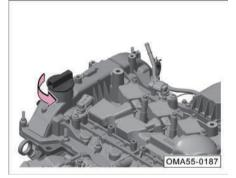
After checking the oil level, if required, add engine oil following the steps below:
