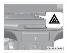
If you press the switch <u>A</u> with ignition in any position, the red indicator lamp on the switch will flash and the hazard warning lamp will be turned on. Press this switch again to turn off the hazard warning lamp.
