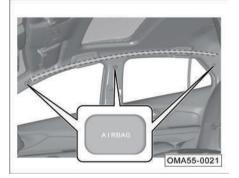
The side curtain airbags are installed in the left and right sides of the roof respectively (as indicated by the dotted dash) marked with "AIRBAG".
