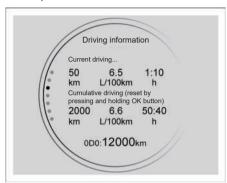
When the vehicle power switch is set to "ON" position, move up or down the "OK" button on the left of the steering wheel to switch to the driving information interface.
