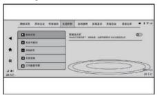
When the vehicle power switch is in the "ON" gear, the system can be turned on or off by clicking the soft button through the AV system "System setting → Body accessories → Exterior light → IHC".
