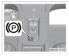
If the service brake fails while the vehicle is in motion, try to continuously pull up the EPB button to achieve emergency braking. Release the EPB button or depress the accelerator pedal and the system exits the emergency braking.
