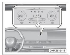
Switch AV system to the control interface of A/ C system, click ION soft button  $\widehat{\ \, }$ 0, soft button indicator lamp will be on, and A/C system will turn on the plasma purifier. It can generate negative ions, effectively decomposing harmful gases such as formaldehyde and benzene in the car, and purifying the air in the car.
