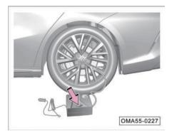
Press the power button to start to inflate the tire, and observe the change in the indicated pressure on the tire pressure gauge. When the indicated pressure reaches the standard pressure, cut off the power to stop inflating the tire.
