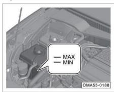
Check whether the coolant level in the expansion tank is between the maximum scale mark "MAX" and the minimum scale mark "MIN".
