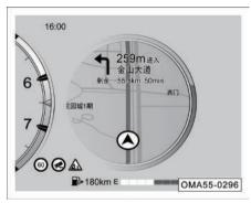
The navigation information can be synchronized to the instrument cluster display after the AV system navigation function is enabled
