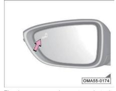
The door open warning system alerts the driver via the yellow indicator lamp  $\mathbb{Q}_{\mathbb{M}}$  on the exterior rearview mirror. The indicator lamp can automatically adjust the brightness according to the external lighting conditions.
