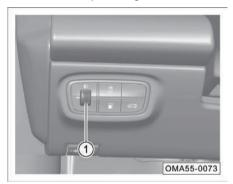
Rotate the knob ① to manually level the headlamp (low beam) at 0, 1, 2 and 3 positions. The level of the headlamp will decrease as the adjustment value increases.
