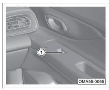
For the operation methods of the passenger's power window control button ①, please refer to the driver's power window control button.
