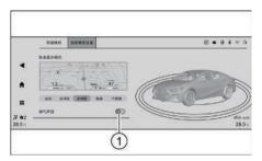
Enter the driving mode-current mode setting through the AVNT interface icon, and select soft button ① to turn on or turn off the exhaust sound according to different driving modes.
