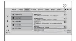
Access the AV system interface, switch to the "System Settings  $\rightarrow$  Driving Assistance  $\rightarrow$  Longitudinal Driving Assistance" interface, and press  $\bigcirc$  soft button on the right of "TSR"  $\bigcirc$  to activate or deactivate the TSR.
