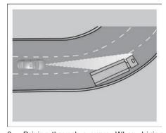
2. Driving through a curve. When driving through a curve, the radar sensor may not catch the vehicle ahead or may not be able to react to the vehicle in the adjacent lane. In this case, ACC may apply the brake to the vehicle in front, reduce the speed, or have no response to the vehicle in front. Depress the brake pedal or manually cancel ACC to exit the ACC system.
