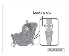
If no means are provided on the child safety seat for securing the seat belt, please install a locking clip on the seat belt.
