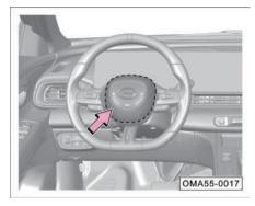
The driver's frontal airbag is installed inside the steering wheel (as indicated by the dotted dash) marked with "AIRBAG".
