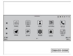
If the vehicle power switch is in the "ON" position or the engine is started, click the "Intelligent Sensing" APP on the multi-function touch screen to access the interface, and activate or deactivate the specific reminder of the corresponding monitoring function through the soft switch.
