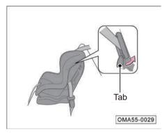
Place the seat belt correctly and push the tab up. Make sure the seat belt is not twisted. When pushing the tab up, pull upward the upper part of the shoulder belt to tension the belt.
