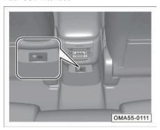
With the ignition in the "ACC" or "ON" position, a device to be charged can be connected directly for charging.
