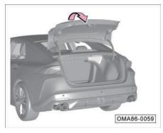
Lower the trunk lid close to the rear bumper cover, and then press the trunk lid firmly to lock it.
