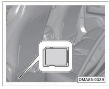
The AVM ECU and TF card are mounted under the driver's seat.
