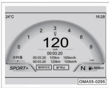
Stopwatch timing can be used to time a road section and will record the latest (last time) and shortest (best time) values in each timing result
