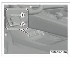
With the ignition in the "ACC" or "ON" position, a mobile device can be connected directly for use.
