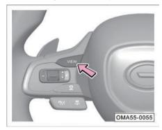
With vehicle power switch set to "ON" position, press "VIEW" button on the left of steering wheel to access the screen of theme setting of instrument panel.
