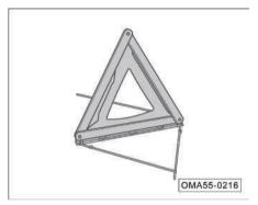
Open the trunk lid, take the warning triangle out and unfold it for use.
