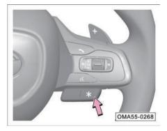
On the right side of the steering wheel, there is a button with the symbol \*. The button has two functional states: press and hold and press. The user can set the press and hold and press corresponding functions at the central control end of the AVN respectively.
