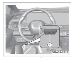
The OBD interface ① for reading the electronic VIN code is located at the lower left rear of the instrument panel, and data such as the electronic VIN code and vehicle status information can be read through the special diagnostic scan tool.
