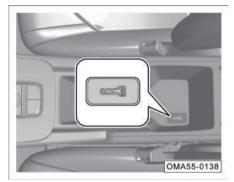
If the smart key battery is low and the instrument cluster display prompts "No key detected", you can try to place the smart key horizontally at the key mark at the bottom of the armrest box, and then press the START/STOP button to switch to the "ACC" or "ON" gear, or press the brake pedal, START/STOP button the backlight color turns green, and press the START/STOP button to start the engine.
