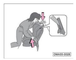
Grasp the shoulder belt near the buckle and pull it up to tension the lap belt. At this time, press the child safety seat with your own weight and push it into the vehicle seat.
