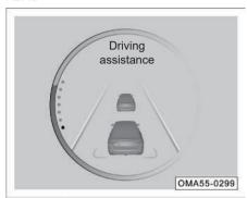
When ADAS function is activated, the corresponding ADAS information, including subject vehicle, left and right lane markings, is displayed. When the forward vehicle is detected, the forward vehicle and the time gap information can be displayed.
