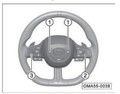
① Horn button: Press dutton to sound the horn; release the button to stop sounding the horn.
