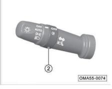
When the ignition is in the "ON" position with the position lamp or low beam turned on, turn the fog lamp switch ② to turn on or off the O\(\xi\$ (rear fog lamp).
