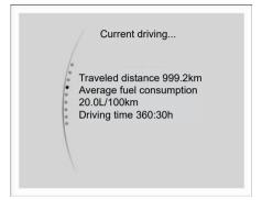
Current trip: It indicates the driving information (trip distance/average fuel consumption/driving time) of the vehicle in a single trip after the vehicle power switch is set to "ON" position, and the single ignition cycle will be reset.
