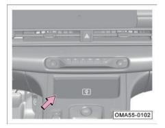
The wireless charging effective zone is in the storage slot in front of the shift lever. To charge the mobile phone, please align its charging coil with the "Qi" logo to ensure the normal charging.
