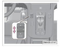
Place the vehicle power supply in the "ON" position. By toggling the driving mode knob up/down, you can click ECO  $\rightarrow$  COMFORT  $\rightarrow$  SPORT  $\rightarrow$  SPORT +  $\rightarrow$  DIY  $\rightarrow$  ECO. The target driving mode is cyclically switched. See => see 181 page
