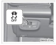
ESP is on by default when the vehicle is running. Press the specific key to turn off ESP. At this time, the specific indicator lamp on the instrument cluster will light up and the alarm message will be displayed.
