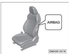
The front seat side airbags are installed in the outboard sides of the driver's seat back and the front passenger's seat back respectively (as indicated by the dotted dash) marked with "AIRBAG".
