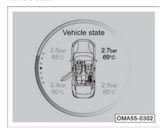
Vehicle status: It contains the tire temperature, the tire pressure, the status of door, engine hood and trunk, as well as seat belt alarm message. This screen will pop up automatically when there is an exception.
