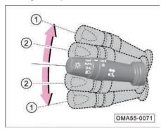
When the vehicle power switch is in the "ON" position, if you turn the lamplight combination switch up or down to the limit position ①, the right or left turn signal lamp will go on, and the corresponding indicator lamp
