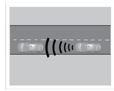
First-level braking: Brake jerk warning is provided when the ego vehicle is approaching the lead vehicle.
