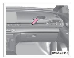
The front passenger's frontal airbag is installed inside the instrument panel (as indicated by the dotted dash) marked with "AIRBAG".
