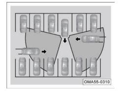
The rear crossing traffic alert (RCTA) system detects blind spots on both sides of the rear of the vehicle via the BSD sensor installed at the rear of vehicle. When the vehicle is reversing, when an approaching vehicle is detected, the system will warn the driver through the visual signal of exterior rearview mirror, instrument alarm sound and the panoramic image.
