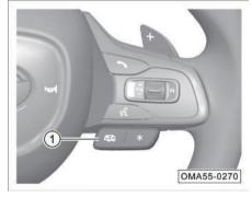
Turn on or off the exhaust sound according to different driving modes with the exhaust sound button switch ① on the right side of the steering wheel.
