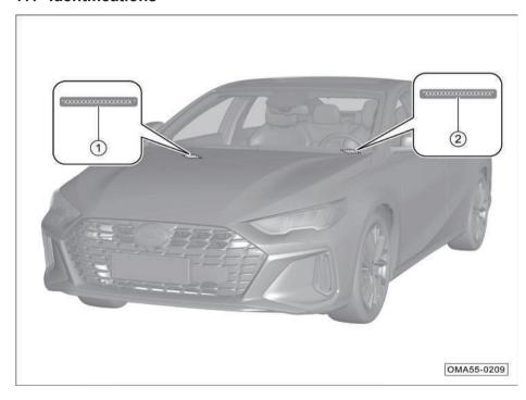
The locations of the vehicle identification number (VIN) is shown in the figure:
