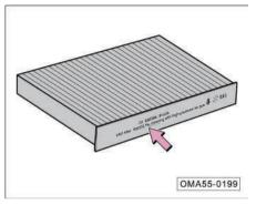
When installing the A/C filter, install it according to the A/C filter down mark.
