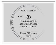
The alarm center is used to save the alarm message. On the alarm message screen, the current state of the vehicle is displayed in the form of texts, pictures, beep sound or others. The driver should always pay attention to checking for alarm message.
