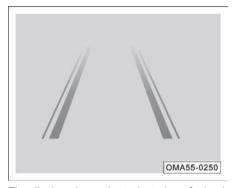
The display shows the trajectories of wheels and the vehicle body.
