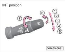
When the vehicle power switch is in the "ON" position, the wiper combination switch can be operated as follows:
