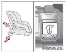
Put the child safety seat on the seat, find the front anchorage ①, and insert the lower guide groove of the child safety seat as arrowed into the front anchorage ① until a click sound is heard.
