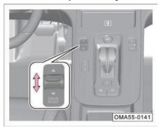
By moving the toggle button up/down, the target driving mode can be selected in the "ECO → COMFORT → Sport → Sport + → DIY ......", jump in gradual circulation, and select the target driving mode.
