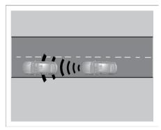
Third-level braking: Full braking is applied automatically when a rear-end collision is inevitable
