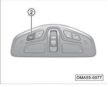
When the dome lamps are off and the switch ② is pressed, the button indicator lamp will come on and all the dome lamps will come on. when the switch ② is pressed again, the dome lamps will go out.
