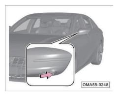
The left/right cameras are respectively installed at the bottom of the left/right exterior rearview mirror.
