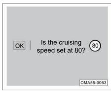
When the pop-up text prompts "Cruising speed set to", "Current speed limit sign" and "OK" appear on the instrument panel:
