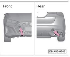
Pry off the towing hook cover in the arrowed position using a slotted screwdriver wrapped with a cloth.
