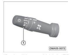
When the vehicle power switch is in the "ON" position, turn the lamplight control switch ① to turn on or off AUTO (automatic headlamp on/ off function)\*, ⇒o∉ (position lamp), and ≝○ (low beam).
