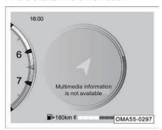
When the vehicle power switch is set to "ON" position, press the button on the right side of the steering wheel to switch to the AV and entertainment information screen. When the AV system is not turned on, the prompt message "Multimedia information is not available" is displayed on the AV and entertainment information screen.
