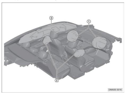
Depending on vehicle configurations, the deployment positions of the SRS are as shown below:
