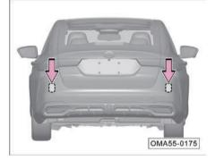
The BSD radar sensors are installed as shown above.
