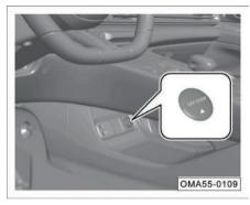
With the vehicle power switch in the "ACC" or "ON" position, after the rear power outlet cover plate is opened, a device to be charged can be connected.
