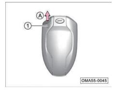
Press the locking button ① and pull out the emergency mechanical key (arrow A).
