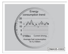
Energy consumption trend graph reflects the fuel consumption information of the last 50km. The update is performed every 1km, and the average fuel consumption of this screen reflects the average fuel consumption of the last 50km.
