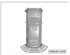
The dynamic view that appears at the upper left of the display indicates the distance of the front and rear of the current vehicle from the obstacle. In the view, the outermost sector is green, the middle & innermost sectors gradually turn to yellow and red. When the vehicle is getting closer and closer to an obstacle detected, the colorful sectors will gradually come nearer and nearer to the vehicle icon
