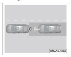
The rear approach alert function monitors the target directly behind the vehicle in real time through the BSD sensor installed at the rear of the vehicle. When the driver drives the vehicle normally on the road and there is a target rapidly approaching in this lane behind, the system will send out an alarm message and a rear-end collision warning signal to the vehicle behind.
