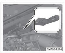
When the engine cools down, check whether the brake fluid level is between the maximum scale mark "MAX" and the minimum scale mark "MIN"
