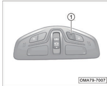
Emergency contact button
